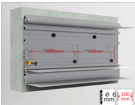
Fastening the profile to the concrete wall
